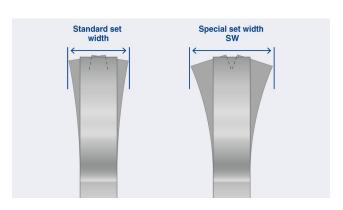
Standard set width compared to special set width SW: The extra wide set increases the free cut of the band saw blade so that there is more clearance to prevent jamming due to released material residual stress.
