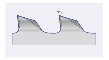
About the profile tooth form: The tooth features a positive cutting angle and a reinforced tooth back.
