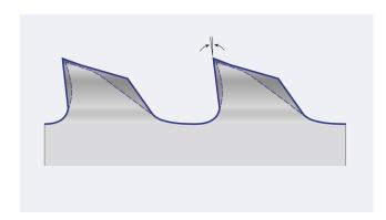
The PROFLEX® PREMIUM M42 is equipped with a special profile tooth form, which have a positive rake angle and a reinforced tooth back. The susceptibility
